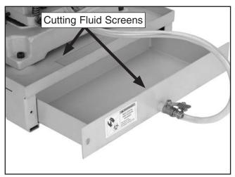
Figure 15. Cutting fluid screens.
